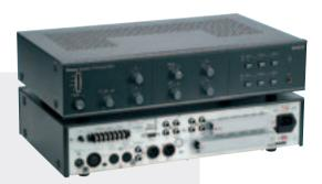
The Plena Multi-Zone Call System provides dual-channel operation (calls and BGM) for 6 zones. The unit is used with Plena Booster Amplifiers. It has 2 call station inputs, each to connect multiple cascaded call stations, a selectable filter for optimizing speech intelligibility, and separate volume control and tone controls for the speech and BGM channels. 6 levels of priority are available for music, microphone, call stations, trigger inputs and the emergency input.
