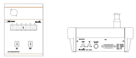
**RM5006** when paging to specific zones is required in which the main rack is located away from the paging station. It is a more economical way of remote zone paging when the number of zones in a setup is small, considering the number of cable used.
