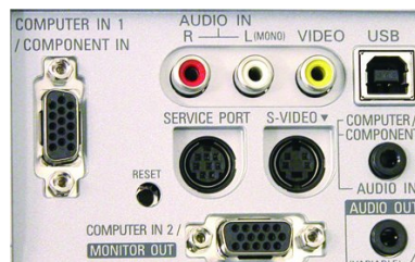
PLC-XU48 Terminal Input Panel (2 inputs, one in/monitor out switchable)
