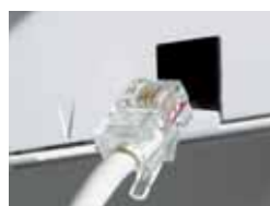
Telephonic plug at the base of the door phone.
